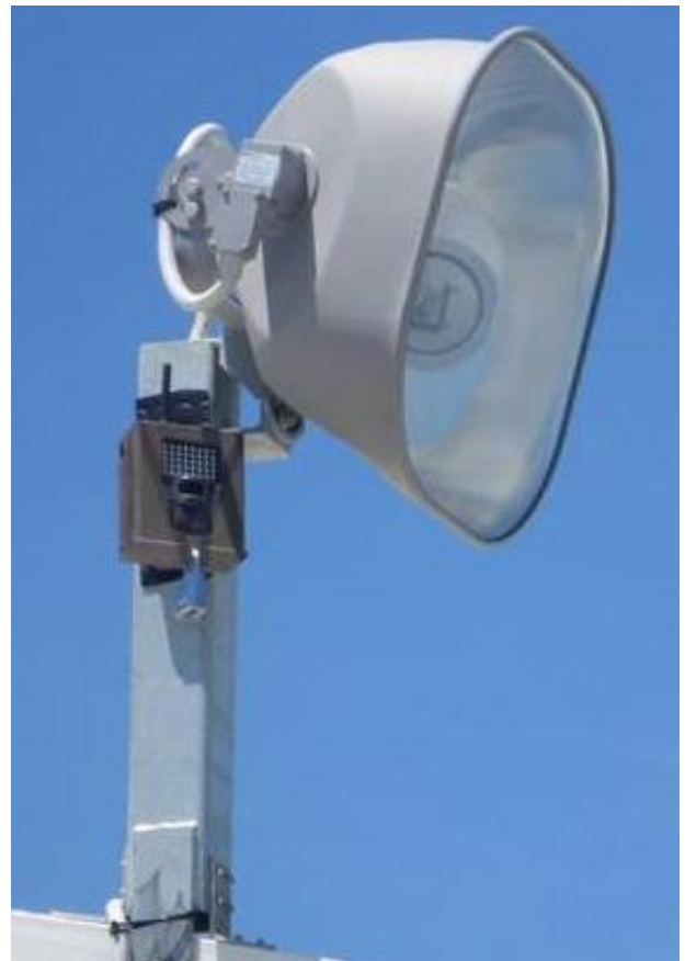
Figure 3.2 Remote imagery unit installation on the light pole on the North Cottesloe Surf Life Saving Club roof
