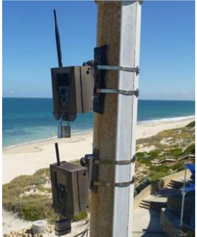
Figure 3.1 Remote imagery unit installation on the light pole in the main beach car park, opposite Overton Gardens
