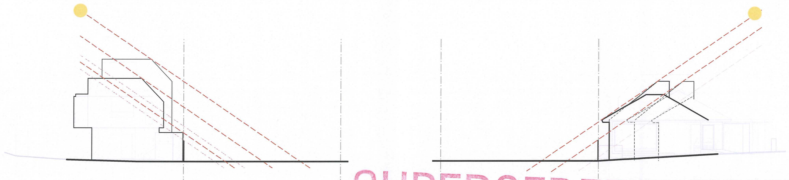
12 NOON WINTER SOLSTICE 21 JUNE; SUN ANGLE: 34.5 DEG OVERSHADOWING SECTIONS 1:200
