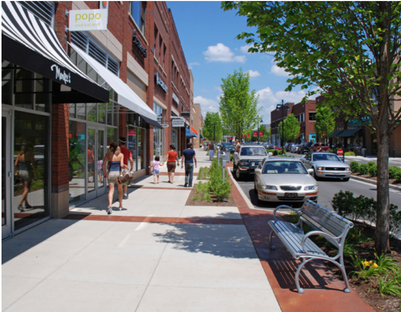
Wider pavements, trees and street furniture make potential obstacles to ram-raiders and enhance the streetscape
